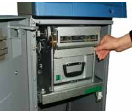
Fig. 5.4 Emptying the Reject Bin
